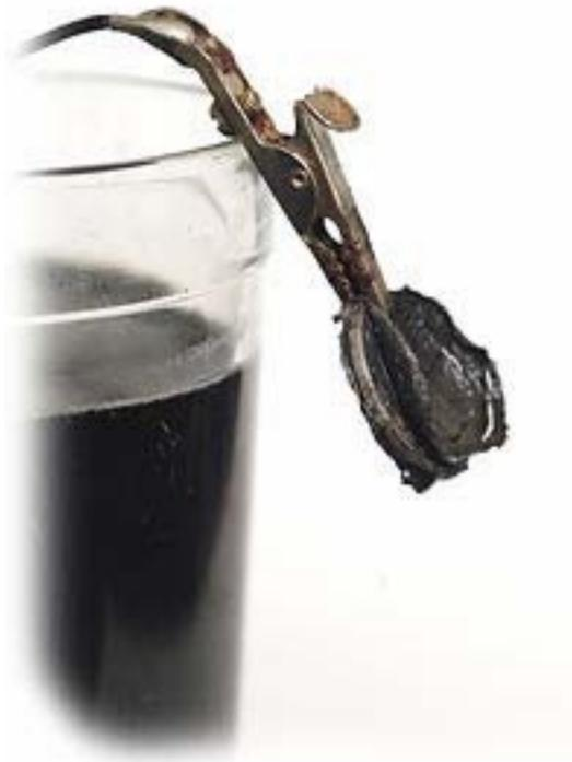
Here's a closer view. To stop the reaction get some baking soda and while rinsing your coin under a faucet, use an old toothbrush and rub some of the baking soda on it. I usually use my fingers, which works good also, but the black will stain your fingers.
