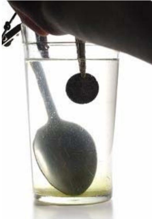
If your spoon starts bubbling you need to switch the alligator clips around. After finding the negative wire, I put a knot on it so I know it goes to the coin.
