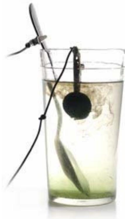
The electrical current is passing through the coin and separating all nonmetallic particles from the coin.
